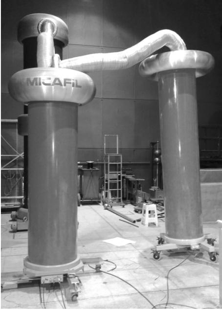
Fig. 5. Intercomparison test between UTE standard capacitor (right) and INTI standard capacitor (left), at the INTI HV Laboratory.
