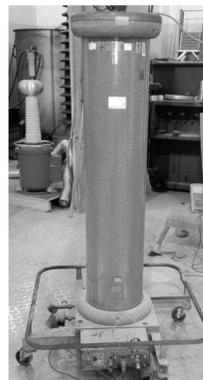
Fig. 1. Typical modern SF<sub>6</sub>-standard capacitor.
