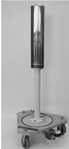
Fig. 3. Internal electrodes of a 100 pF, 100 kV, gas compressed capacitor.
