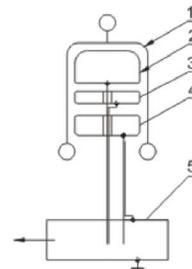
Fig. 2. Internal diagram of a standard capacitor. 1—High voltage electrode. 2—Main-capacitor low-voltage-electrode. 3—Shield electrode. 4—Auxiliary-capacitor low-voltage electrode.
