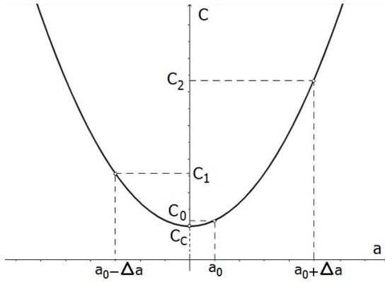
Fig. 4. Relation between capacitance and axes eccentricity.
