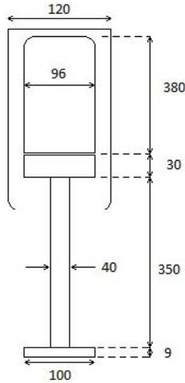
Fig. 6. Electrode dimensions in millimeter of a 100 pF, 100 kV, capacitor.
