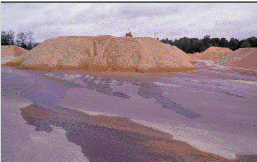
PAVED, SLOPED STOCK PILE AREAS SAVE MONEY
